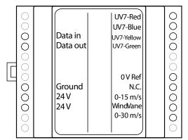
LED "Data in" flashing: data transfer OK. LED "Data out" flashing: microprocessor is working properly.
